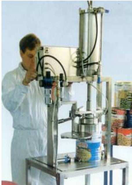
Can opening: Punching out of the can lid
