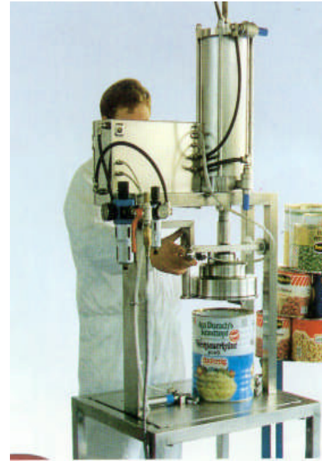
Ejection of the can lid into the emptied can
